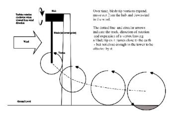
Drawing 1: Vortex creation from a single wind turbine blade at the lowest point of travel (mast interference has been ignored)
