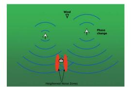
Figure 19: Noise from 2 turbines under slightly different conditions moving Heightened Noise Zones
