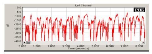
Figure 3: Pulse pattern from an operational wind farm
